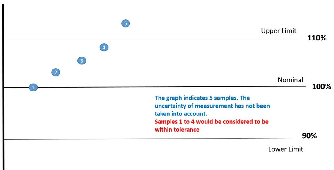
Fig 2.0 Set of samples with 4 samples within tolerance
